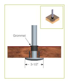
Verify Counter Thickness or Under-Counter Installation Depth in Inches
