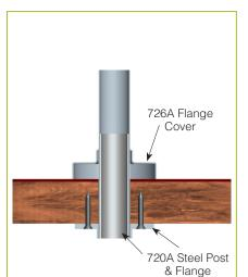
Under-Counter Installation 720A: Steel Post and Flange w/out Flange Cover
