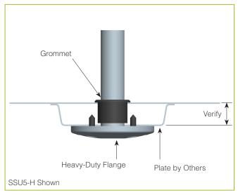
Verify Counter Thickness or Under-Counter Installation Depth in Inches
