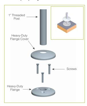
For Millwork Counter MW2: Narrow Flange
