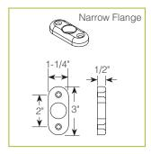
For Millwork Counter MW1: Heavy-Duty Flange
