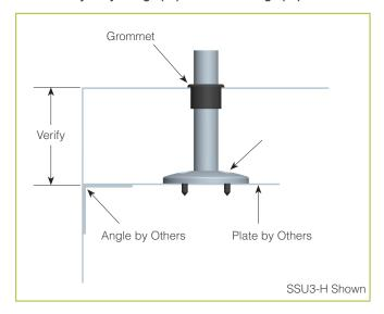
For Stainless Steel Counter (requires under-counter reinforcement and access) SSU5: Heavy-Duty Flange (-H) or Narrow Flange (-N)
