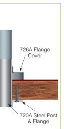
**Under-Counter Installation 720A:** Steel Post and Flange w/out Flange Cover
