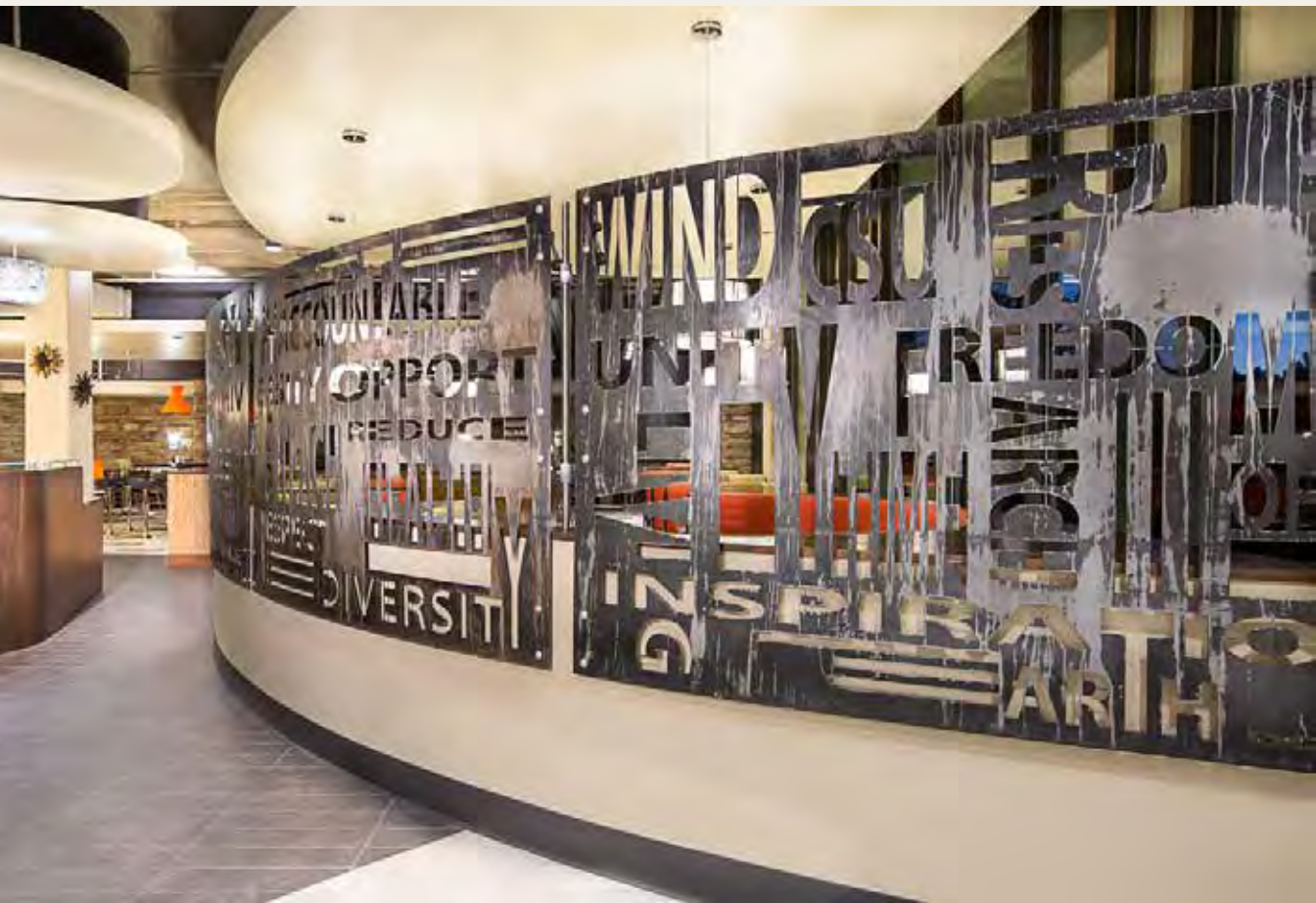
This metal wall was laser-cut in-house and BSI developed a technique to “age” the metal. It’s also mounted with XGuard food guard brackets to match the servery.
